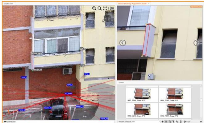
We can select points and vertexes from **graphic view** or directly from the photos from **Stereo Drawing** panel.
