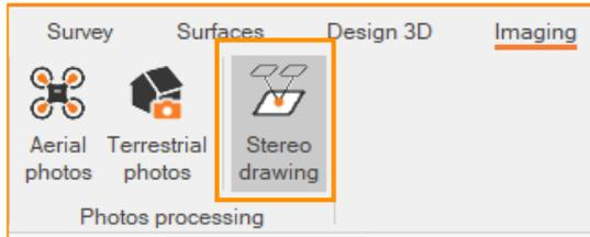
Based on analytical photogrammetry process we can use the Stereo Drawing function for the manual computation of coordinates in 3D space
